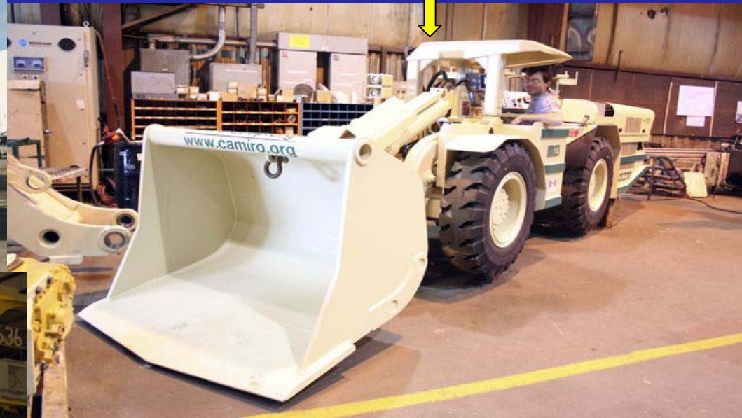
Hybrid diesel electric loader manufactured by Mining Technologies International
